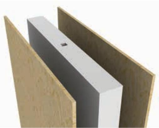
Structural insulated panels are high-performance building panels used in exterior walls, roofs and floors. The panels are made by sandwiching a core of rigid foam insulation between two skins of wood structural panels, typically oriented strand board (OSB).
